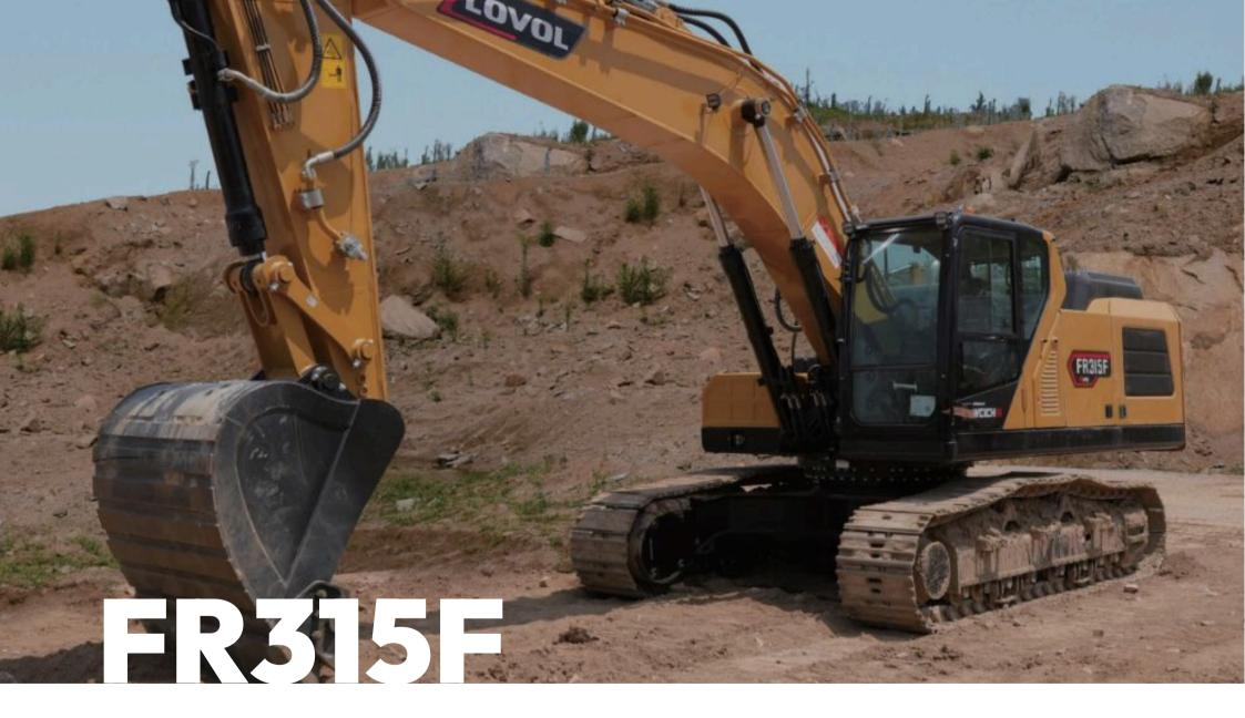
Rated Power Operating Weight Bucket Capacity 228kW/2000rpm 31000kg 1.7m3
